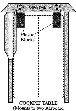
(Mounts to two starboard blocks that are attached to metal plate)
